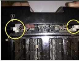
Detach the cable that connects the toaster to the circuit board, in both control panels.
