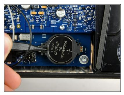
Use the tip of a spudger to pry the PRAM battery out of its holder.
