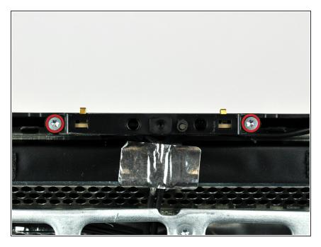
Remove the two 9 mm T8 Torx screws securing the camera board to the rear case.
