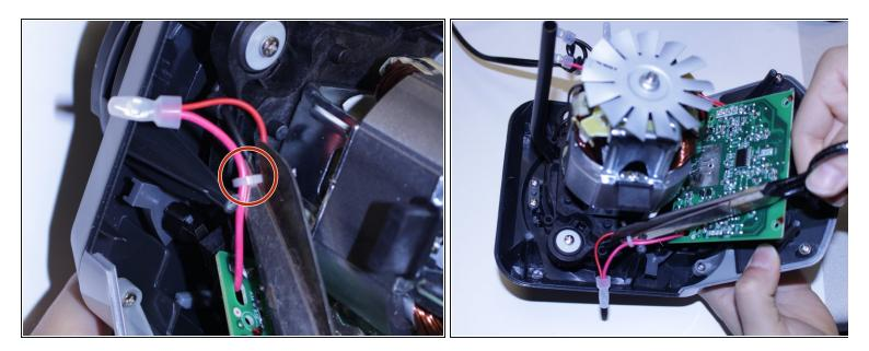
• To give the circuit board further range of motion, remove the pictured zip ties holding the cables.
