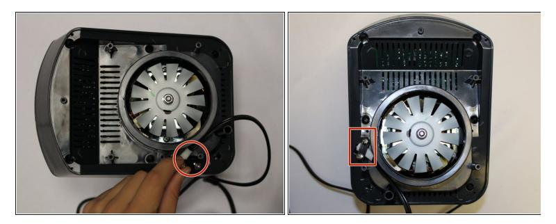
• Using the Phillips #1 screwdriver, remove the two screws (5 mm long, 3 mm wide) holding the power cord onto the motor cover.
