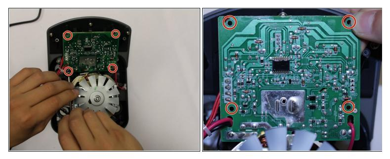
Using the Phillips #2 screwdriver remove the 4 screws (10mm long, 5mm wide) on the circuit board.
