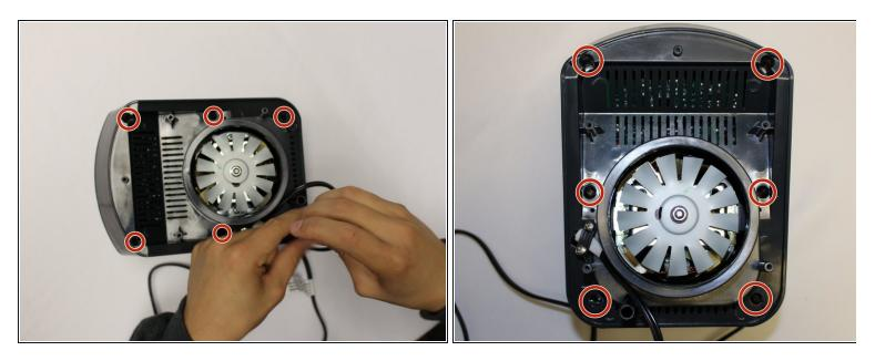
Using the Phillips #1 screwdriver, remove the 6 screws (13 mm long, 6 mm wide).
