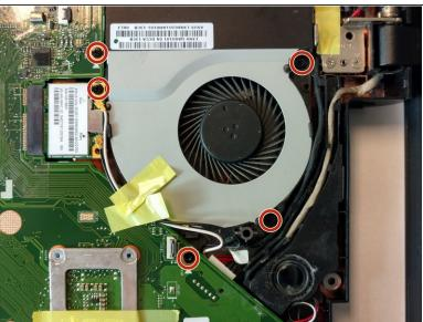
Using the Phillips #0 Screwdriver, remove the nine 2mm screws at the marked locations.
