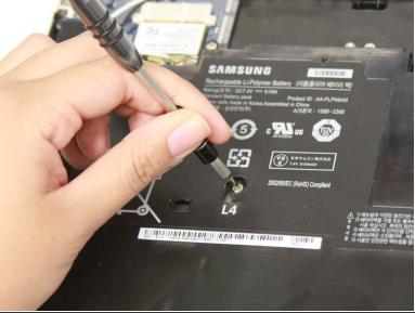
• Remove the four 3 mm screws using a Phillips #000 screwdriver.
