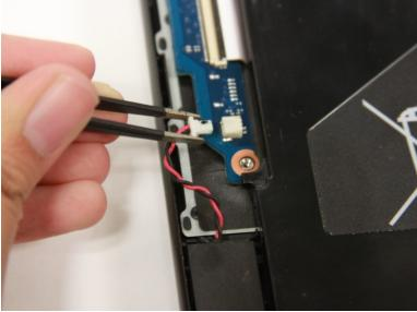
• Use a blunt precision tweezer to remove the speaker cord from the R.A.M.
