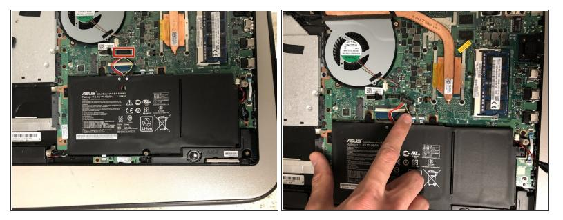
Disconnect the wires at the top of the battery by lifting on the tabs protruding out of the plastic frame.
