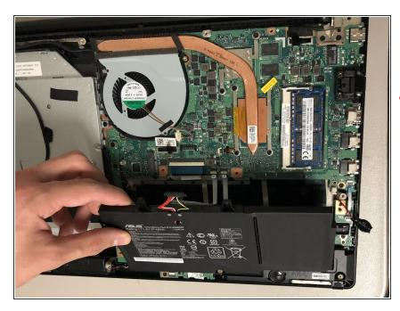
• Gently lift out the battery by the side closest to the motherboard first.
