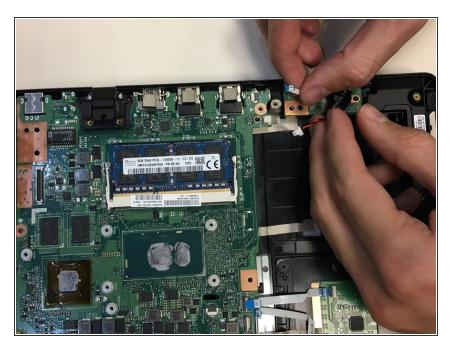
• Move to the top of the motherboard and unplug the two cables that are connected.
