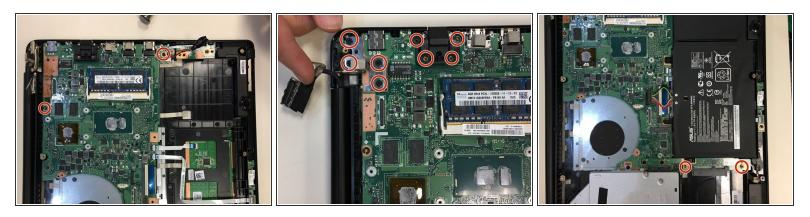
• Next remove the screws at the top and bottom of the motherboard.
