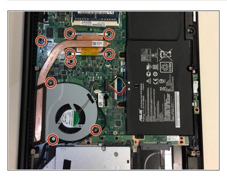
Next you will be removing the cpu fan. Begin by removing the nine screws holding it in place.
