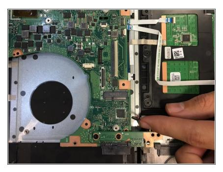
Move to the bottom of the motherboard and unplug the single cable near the battery.
