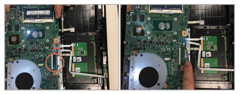
Underneath the battery are 3 cables plugging into the motherboard, 1 wide one and two small ones. Lift the white tabs above them up, and then slide them out.
