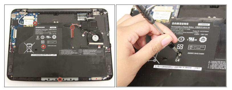
Remove the four 3 mm screws using a Phillips #000 screwdriver.
