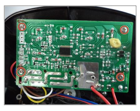
Remove 4 screws (11mm, 4mm head) connecting the circuit board to the base.
