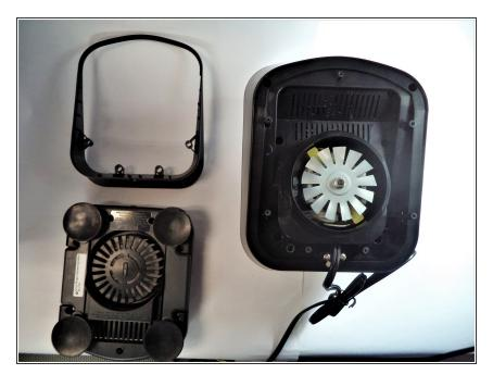
Carefully remove the second layer from the base. You will not need a screwdriver for this step.
