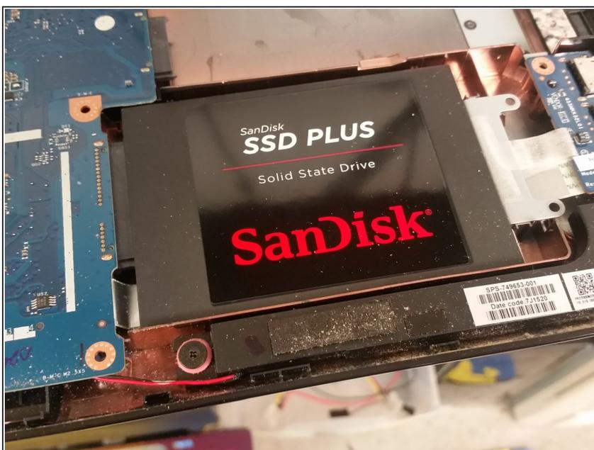
ⓘ Normally, there will be two screws holding the hard drive (or, in this case, solid state drive) in, but in this case, the screws are missing, and the SSD slid out from the connector. The computer wasn't showing any drive, and hence, it was brought in for me to repair.
