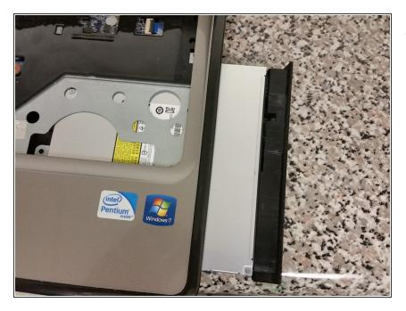
Simply slide out the optical drive, the screw holding it was removed in the last step.
