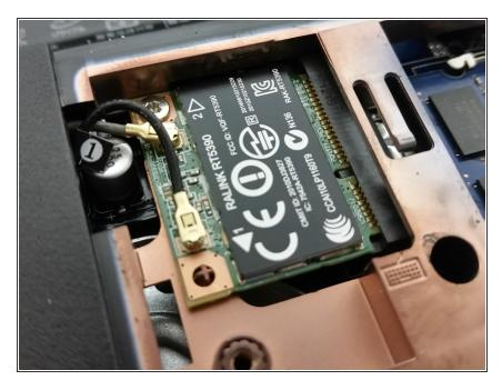
• In order to remove the motherboard, you must remove the wireless card. Unscrew the single silver Philips screw holding the wireless card, pop each antenna off its connector with your fingernails, pull the wireless card out, and set it aside.
