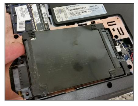
Simply pull the hard drive upwards and out, there are no screws. Be sure to disconnect the connector from the board.
