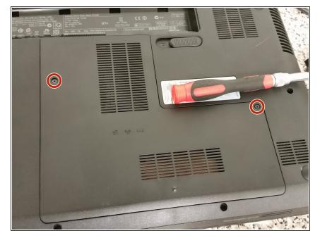
Flip the laptop bottom-upwards, and remove the two screws securing the bottom cover, and pull the bottom cover off.
