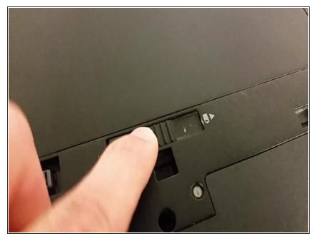
• With the back of the laptop facing towards you, simply push the battery latch to the right, and out comes the battery.
