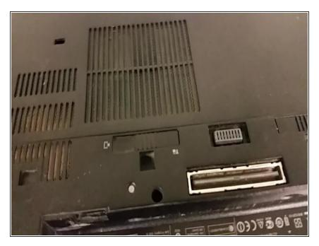
Push the latch to the left like shown in the video, and then help the bottom cover off, like in the attached video.
