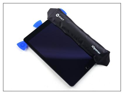
Reheat the iOpener and lay it over the right edge of the display to loosen the adhesive underneath.
