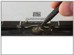
• Continue working the tip of the spudger around the edge of the gasket until the gasket is fully separated from the front panel.
