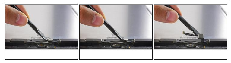
• Use the flat end of a spudger to peel up the Home Button ribbon cable and Touch ID control chip.
