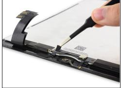
• Peel up the tape covering the Home Button ZIF connector.
