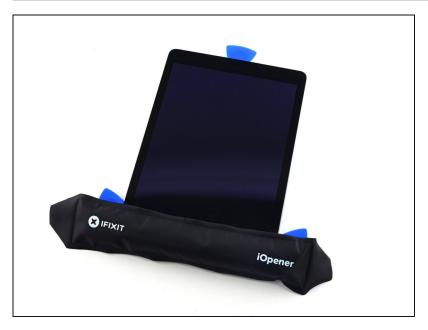
• Use the iOpener to apply heat to the bottom edge of the iPad.
