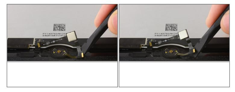
• Peel up the remaining corner of the Home Button ribbon cable.
