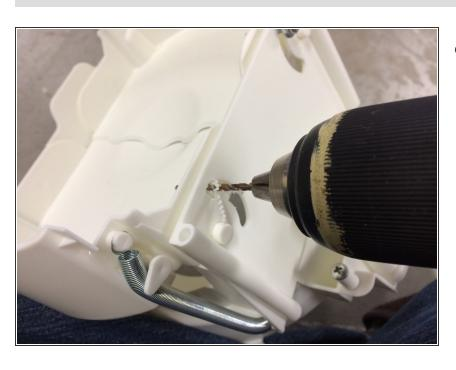
Use a 1/8" drill bit to drill through the center of the original tab location until you have a nice, clean hole.
