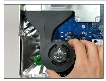
• Gently lift the CPU fan out of the rear case.
