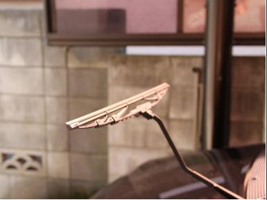
Rotate the wiper blade assembly so the replaceable blade faces outward.
