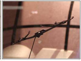
After removing the clasp, pull the blade from the wiper arm.
