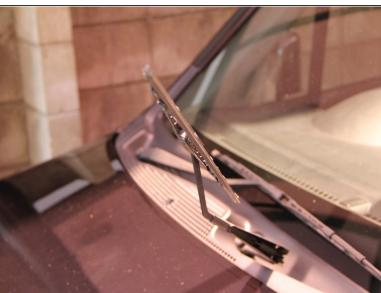
Grab the windshield wiper at the base and lift in a counter-clockwise motion around the hinge, lifting the blade from the window.
