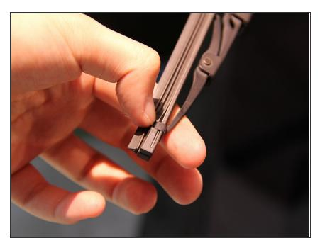
Reattach the clasp by sliding it back over the edge of the wiper blade.
