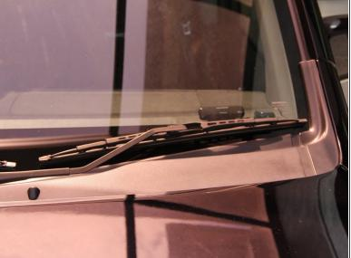
Rotate the wiper arm clockwise around the hinge until it rests on the windshield.
