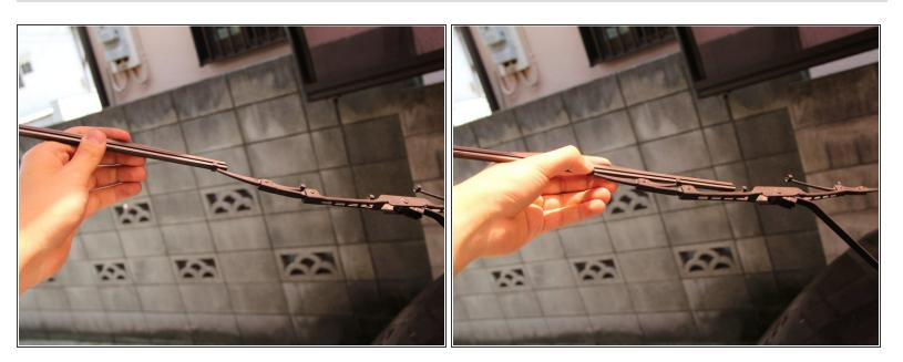
Insert the new blade by sliding it back into the slots on the wiper arm.
