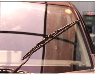
Return the windshield wiper blade back to its original orientation.
