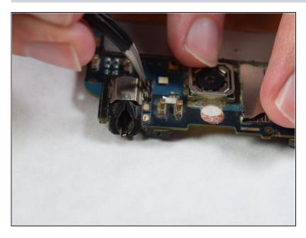
Using tweezers, remove the adhesive tape around the headphone jack.
