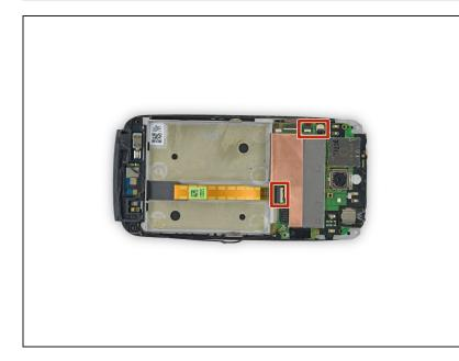
Repeat the procedure from steps 19 and 20 to remove the cables from the remaining ZIF connectors.
