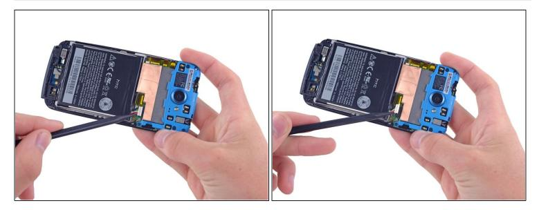
• Using the pointed end of a spudger, lift the battery cable and release the connector.
