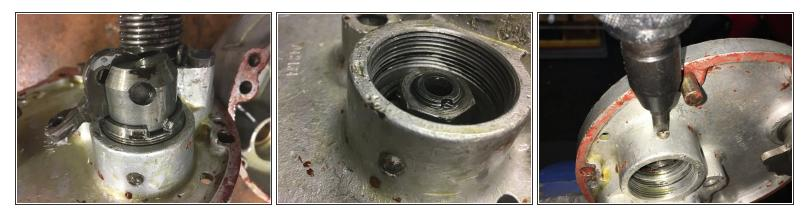
• The clutch actuator is held in place with a threaded ring. Ideally, you would use a C-spanner to remove it, but access is so restricted that you will probably need to use a drift and hammer...
