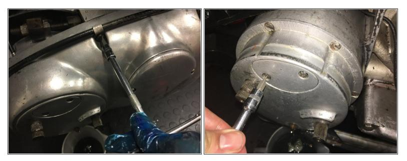
• Undo the four screws holding the right side cover on and remove it.
