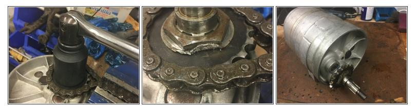
• Fit the output sprocket, tab washer and nut.
