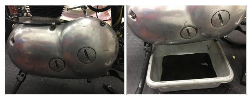
• Remove the six screws holding the primary drive cover on.
