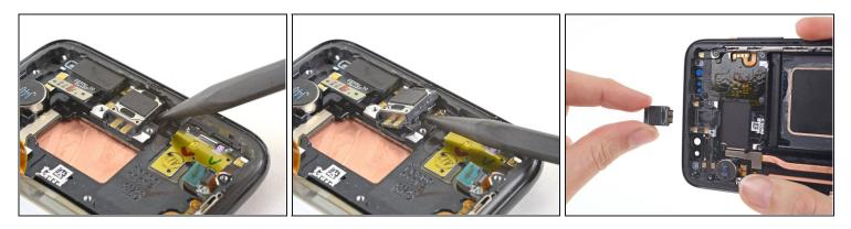
• Insert the pointed end of a spudger into the small slot on the side of the earpiece speaker. Use the spudger to pry the speaker out of its slot.
