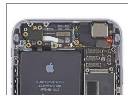
• Remove the single 1.2 mm Phillips screw securing the antenna interconnect cable to the logic board.
