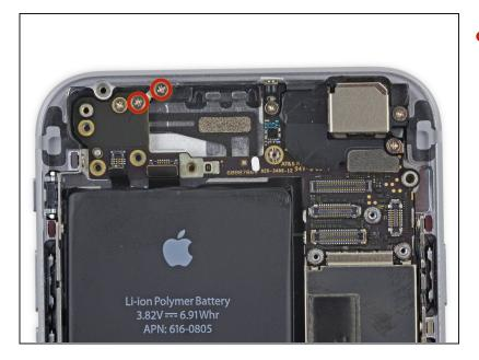
Remove the two 1.6 mm Phillips screws from the grounding bracket.
