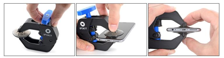
(i) The next two steps demonstrate the <u>Anti-Clamp</u>, a tool we designed to make the opening procedure easier. **If you aren't using the Anti-Clamp, skip down three steps for an alternate method.**
