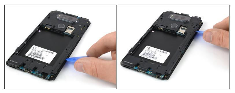
Slide the opening pick along the mid frame and flip it sideways to open the plastic clamps holding the motherboard cover in its place.
