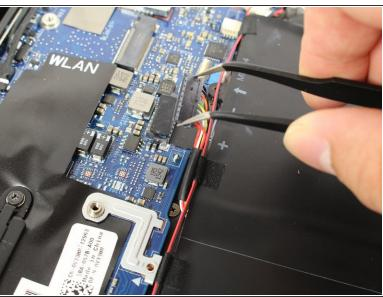
Pull the battery cable connector towards the battery to disconnect it from its socket.
