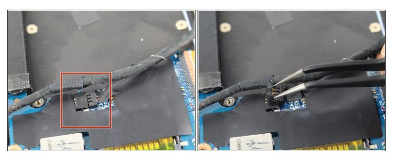
Use tweezers to detach the black cable connector out of its socket by pulling it to the right.
