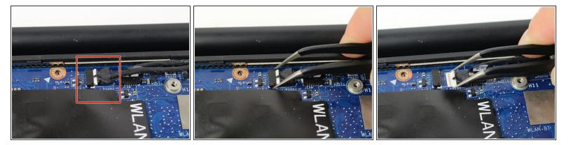
Use tweezers to gently detach the black and white cable connector out of its socket by pulling it to the right.
