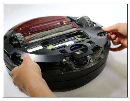
Pull up on the bottom panel to remove.
