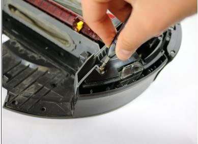
• Using a Phillips #1 screwdriver, remove the four 10 mm screws shown.
