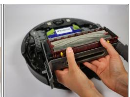
Remove the cleaning head by grabbing the two protruding tabs as shown, and pulling straight up.
