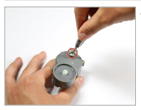
Remove the 10mm Phillips #1 screw holding down the lid of the side brush motor case.
