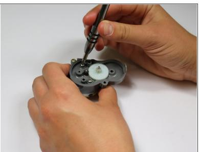
Remove the three 10mm Phillips #1 screws.
