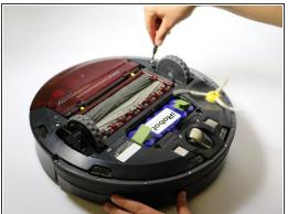
Remove two 15mm Phillips #1 screws beneath each side wheel.
