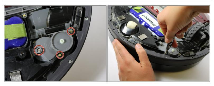
Remove the three 10mm Phillips #1 screws holding down the side brush motor case.
