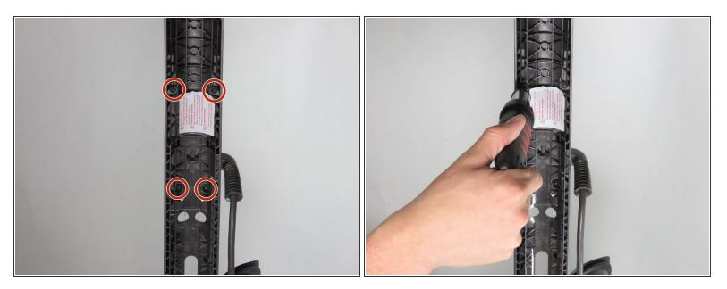
• Remove the four 15mm screws behind the power button using a Torx T15 screwdriver.
