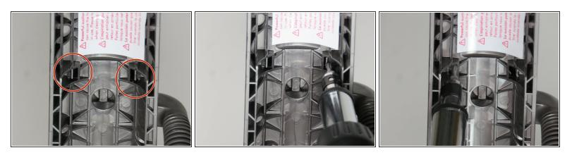
Use a spudger to push the two clamp tabs behind the power button towards the middle of the vacuum.
