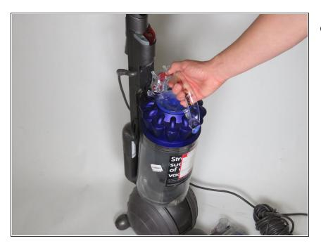
Press the red release button and pull the canister up and away.
