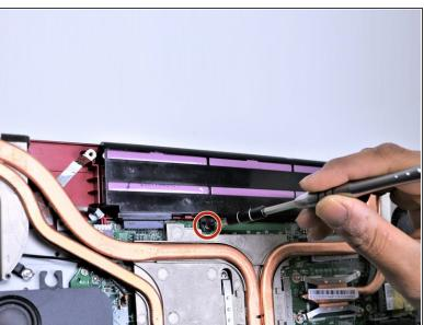
Unscrew the single 5.5mm Phillips #1 screw keeping the battery secure.
