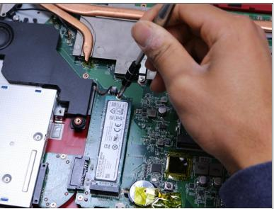
Remove the single 5.5mm Phillips #1 screw attaching the SSD to the laptop.
