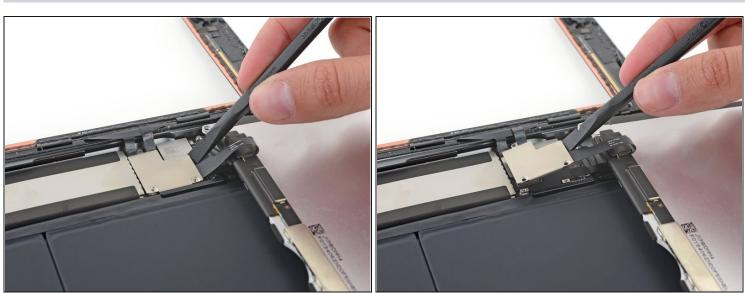
• Use the flat end of a spudger to gently pry the display cable bracket straight up from the logic board.
