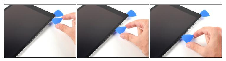
• Insert a new opening pick and slide it to the middle of the iPad's right edge.
