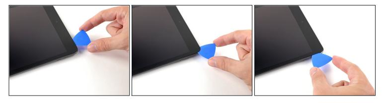
• Rotate the pick around the top-right corner of the device to separate the adhesive.
