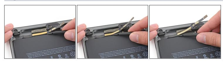
Slide the flat end of a spudger under the headphone jack cable to free it from the adhesive securing it to the rear case.
