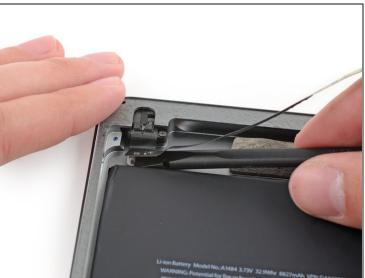
• Continue to slide the spudger under the end of the headphone jack cable to remove the last of the adhesive.
