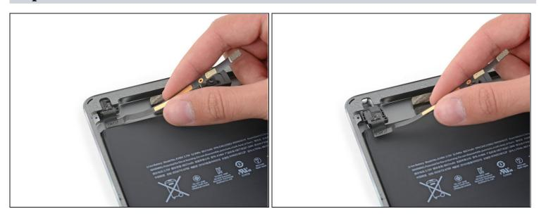
• Use the headphone jack cable to gently remove the headphone jack from its recess in the case.
