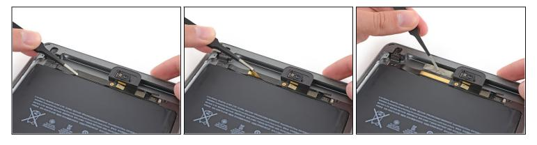
• Lift the tape covering the headphone jack cable toward the top of the iPad to free the cable for removal.
