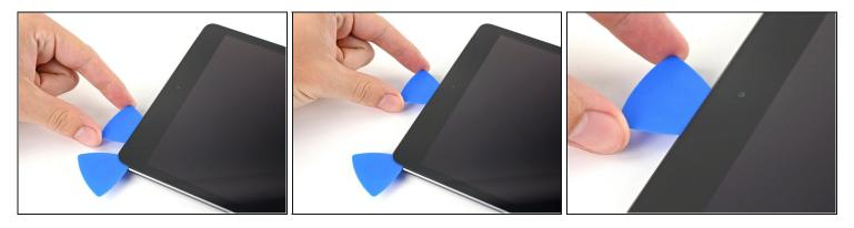
• Slide the opening pick along the top edge of the device, stopping just before you reach the front camera.
