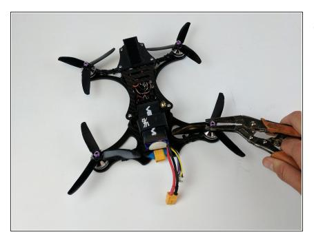
• With your set of pliers loosen and remove the four bolts holding the propellers to the motor.
