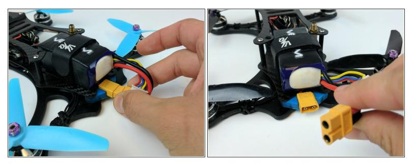
• Unplug the power cable of the drone to eliminate unnecessary mishaps.
