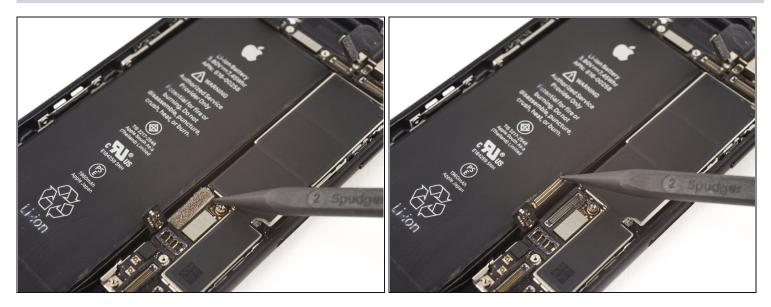
• Use the point of a spudger to disconnect the lower cable connector.
