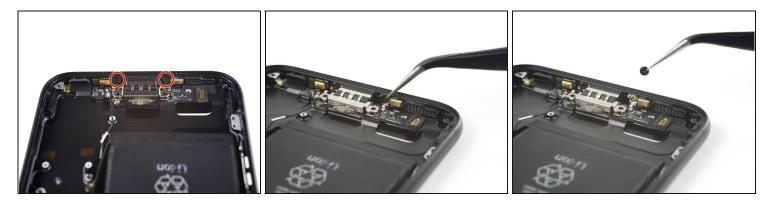
• Remove the two stickers covering the screws that secure the lightning connector to the bottom of the rear case.
