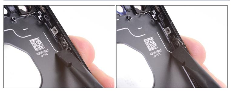
• Push the lower end of the power button bracket up off of peg securing it.
