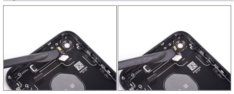
• Use the blade of a Halberd spudger to separate the adhesive holding the microphone to the rear case.
