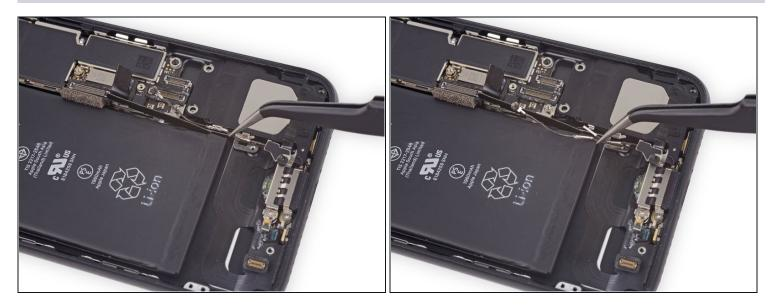
Use tweezers to remove the antenna cables from the clip on the speaker.
