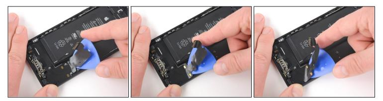
• Continue to slide the pick towards the lightning connector to further separate the assembly from the rear case.
