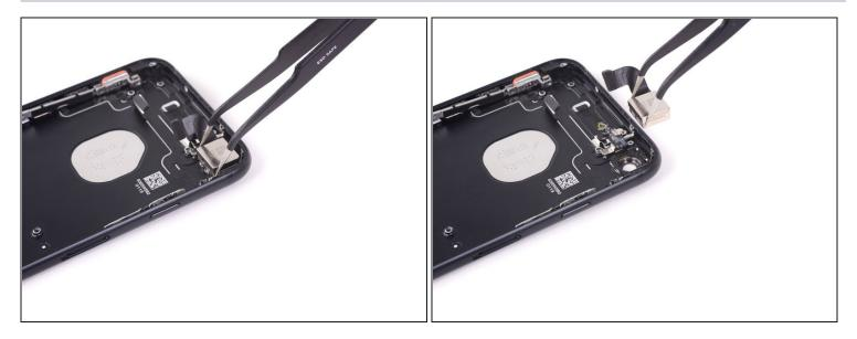
• Use a pair of tweezers to remove the rear-facing camera.
