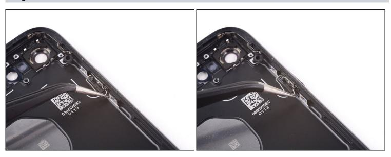
• Pull the clip towards the bottom of the phone and lift up to free it from the bracket.
