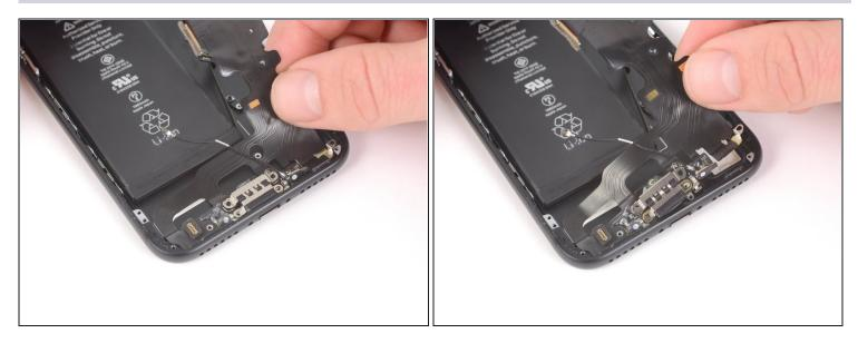
• Gently pull the lightning connector out of its hole on the rear case.
