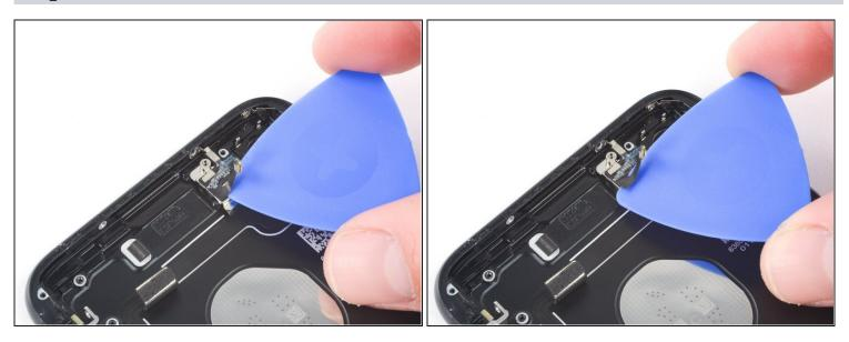
• Moving from power button side of the phone, use an opening pick to separate the adhesive holding the antenna flex cable to the rear case.
