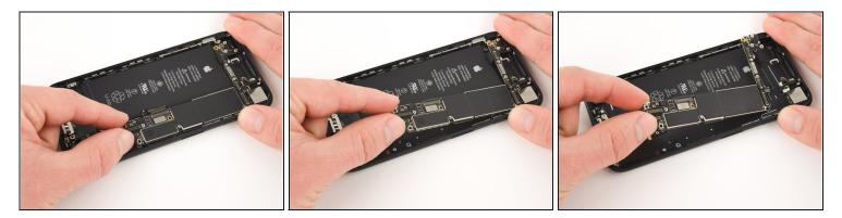
Lift the battery connector end of the logic board and pull it up and out of the rear case.
