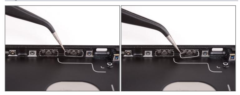
• Pull the volume button clip towards the bottom of the phone to free it from the bracket.
