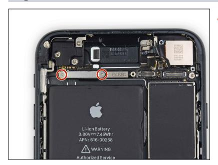
• Remove the two 1.2 mm tripoint screws securing the upper cable bracket.
