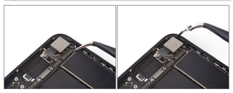
• Use tweezers to gently bend the logic board grounding bracket out of the way.
