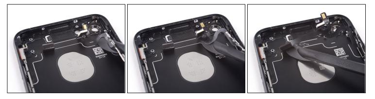
• Continue to move the blade of the halberd spudger underneath the power and volume control cable.
