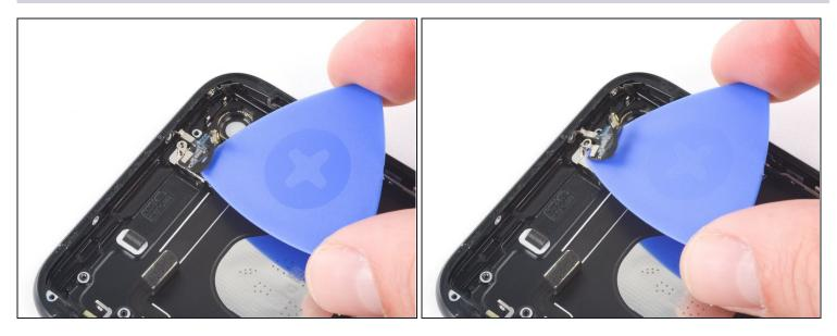
• Slide the point of an opening pick underneath the antenna flex cable towards the top of the phone, separating the remaining adhesive.
