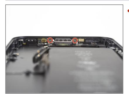
Remove the two 1.3 mm Phillips screws from the rear case.
