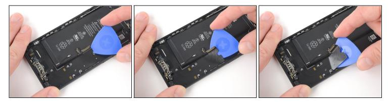
• Starting from the middle of the phone, slide an opening pick underneath the lightning connector to separate it from the rear case.
