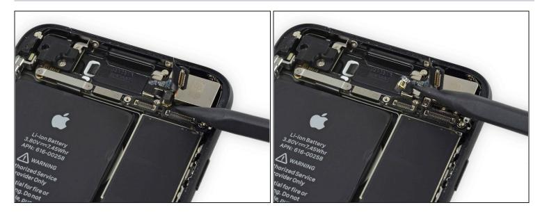
• Use the pointed end of a spudger to pry up and disconnect the antenna bus connector, just left of the rear camera module.
