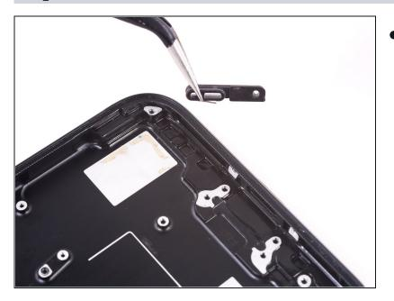
• Remove the right rubber speaker vent from the rear case.
