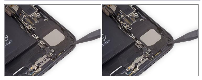
• Use the tip of a spudger to slide the speaker assembly towards the logic board and off of the rear case.
