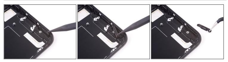
• Use the point of a spudger to push the left rubber speaker vent out of the rear case.
