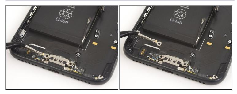
• Remove the spring contact from the lightning connector.
