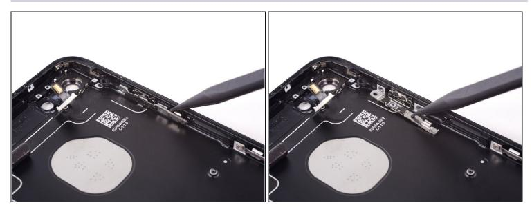
• Gently fold the power button module from the edge of the rear case.
