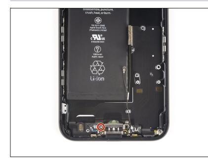
• Remove the 2.9 mm Phillips screw from the lightning connector.
