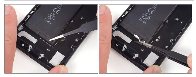
• Use a pair of tweezers with blunt tips to peel back one of the adhesive strips on the lower edge of the battery.
