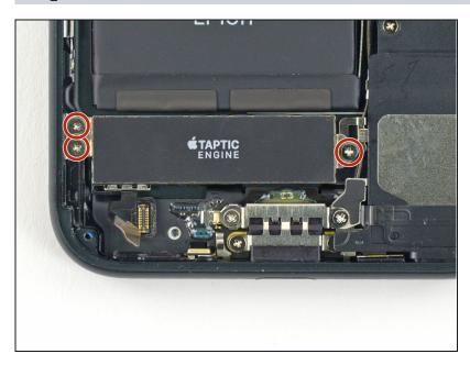
• Remove the three 1.6 mm Phillips screws securing the Taptic Engine to the rear case.
