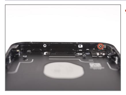
• Remove the 1.5 mm Phillips screw securing the grounding bracket.
