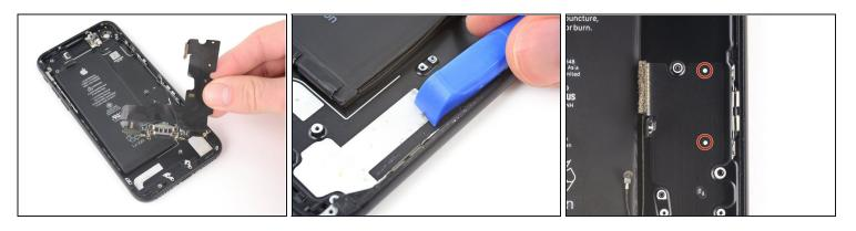
• Remove the lightning connector assembly.
