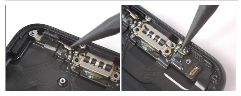
• Use the pointed end of a spudger to separate the two microphones from the bottom of the rear case.
