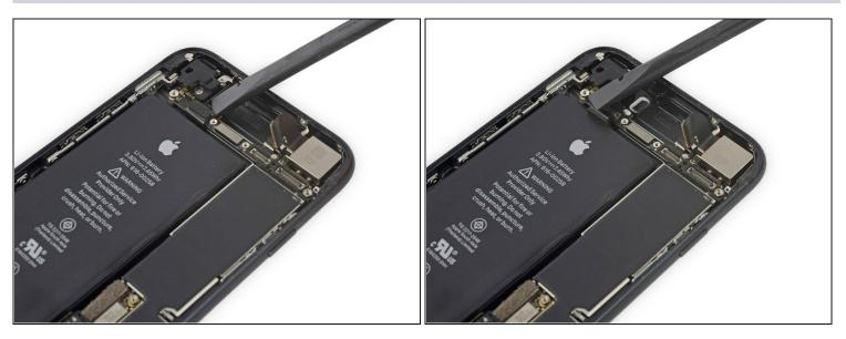
• Use the flat end of a spudger to disconnect the upper cable connector.
