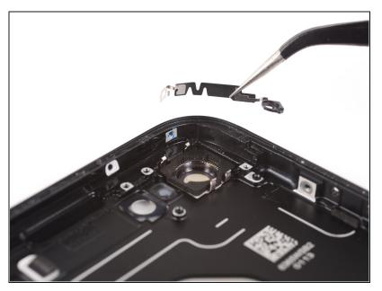
• Remove the grounding bracket.
