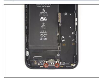
• Remove the two 1.6 mm Phillips screws securing the lightning connector cable in place.
