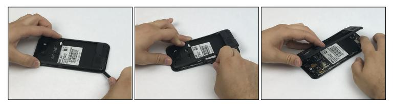
• Now that all the screws have been removed, use a plastic opening tool to carefully pry at each of the corners until loosened.
