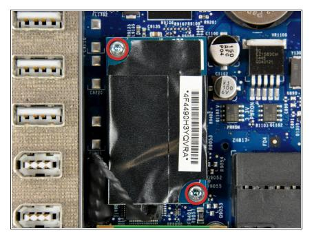
Remove the two 5.5 mm T6 Torx screws securing the modem to the logic board.
