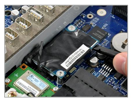
Pry the modem straight up from its top edge to disconnect it from the logic board.
