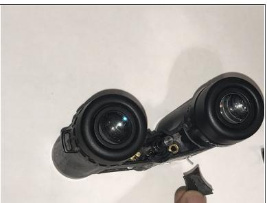
Locate the panels in front of the binoculars between the middle axle and the viewing lens and simply pry them off with your fingers
