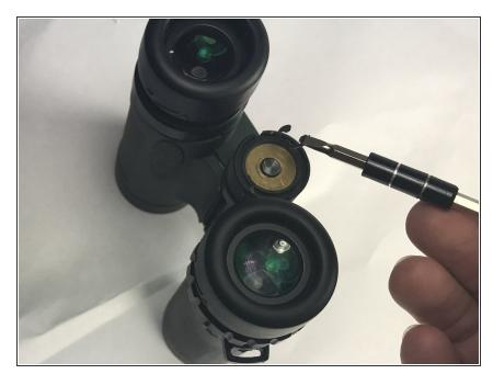
Use a magnetic pickup tool or magnetic screwdriver head to remove the guard. The guard should come right off without much resistance.
