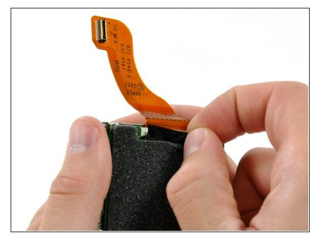
If present, remove the small piece of black tape covering the ribbon cable connector.
