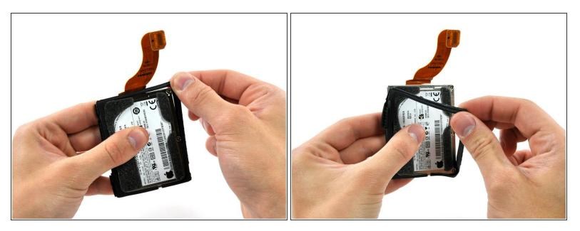
• Peel the rubber shock isolator off the perimeter of the hard drive.
