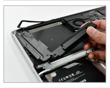
Lift the subwoofer and right speaker assembly out of the upper case.
