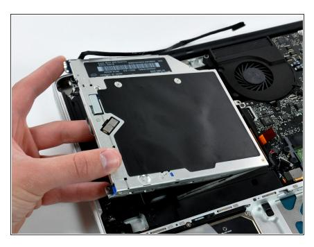
Lift the optical drive from its left edge and pull it out of the computer.
