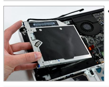
Lift the optical drive from its left edge and pull it out of the computer.
