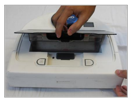
Looking straight at your Neato machine lift up the black plastic piece where filter is located.
