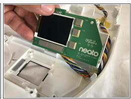
There are two 0.5cm #1 Phillips screws holding the LCD screen to the top cover. Remove these screws to lift screen off the cover.
