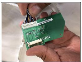
With the two screws removed you may lift the screen off the cover. Carefully remove the connector from the screen by pulling on the connector.
