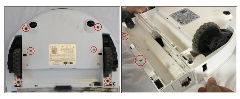
• Eight 13mm T10 screws on the underside of the Botvac hold the casing together. These screws are not self-retained so make sure that you don't lose them in the disassembly process.
