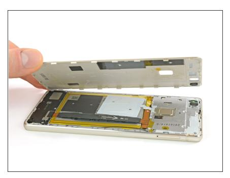
When the back cover is freed from the adhesive you can pop it off by hand completely.
