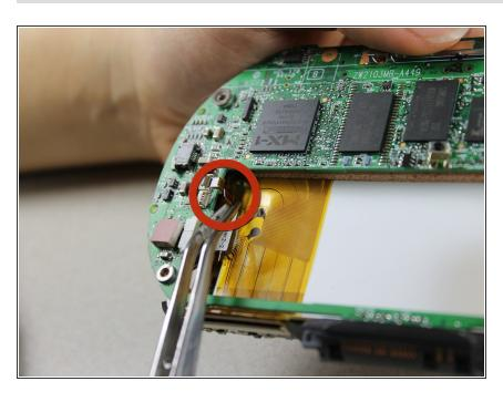
Disconnect the 2 brown wire-tape ends from the left side of the battery slot on the motherboard using tweezers.
