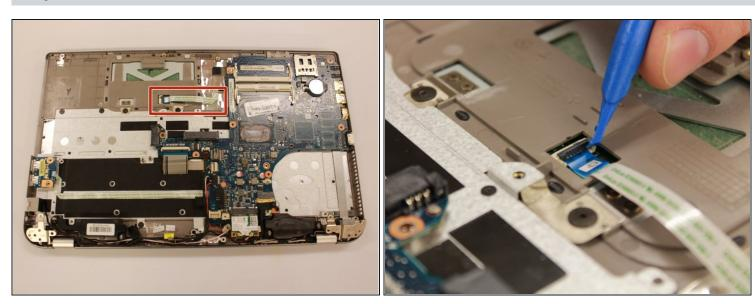
Using a plastic opening tool, remove the CP Tab that was plugged into the touchpad.
