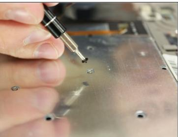
Using the #J000 screw head, remove 4 small (1.67 mm) screws.
