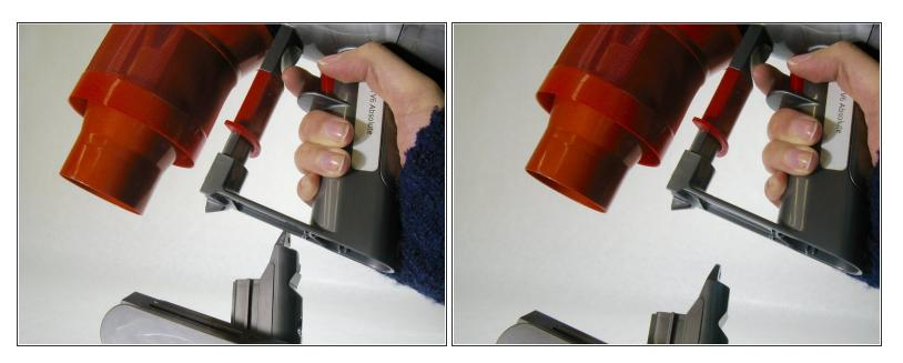
Pull the battery pack down and away from the device.
