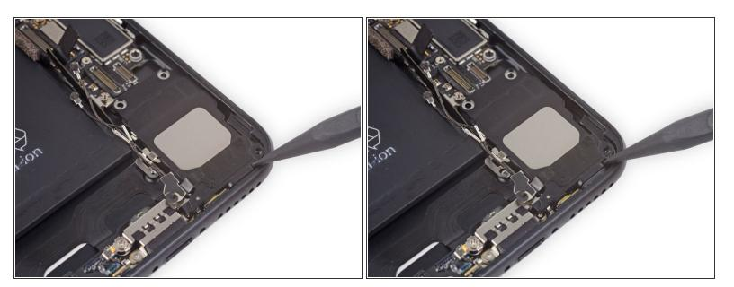
Use the tip of a spudger to slide the speaker assembly towards the logic board and off of the rear case.
