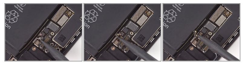
Use the point of a spudger to lift the two antenna cable connectors up off of the sockets on the logic board.
