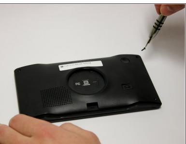
Using the T4 Torx screwdriver, unscrew all four of the screws (1/4 inch, 6.35 mm) from the back panel of your device.
