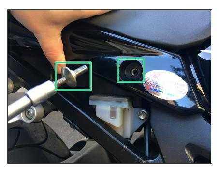
• First you have to remove the screws with an Imbus key (size 4) on the left and right side.
