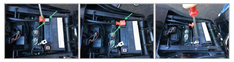
A Before the battery can be reconnected all power consumers (light, ignition, etc.) must be shut off.
