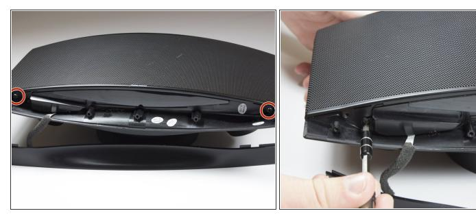
• Use a TR 10 screwdriver to remove two of the 10mm screws that secure the speaker grille.
