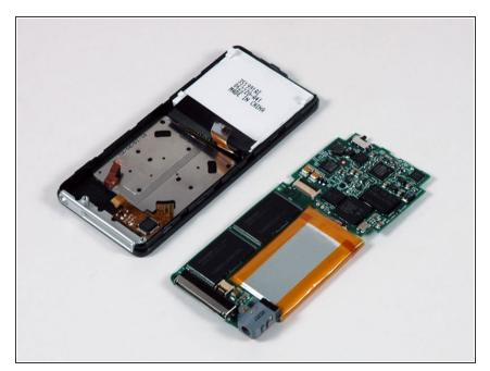
The logic board and battery are now free from the iPod.
