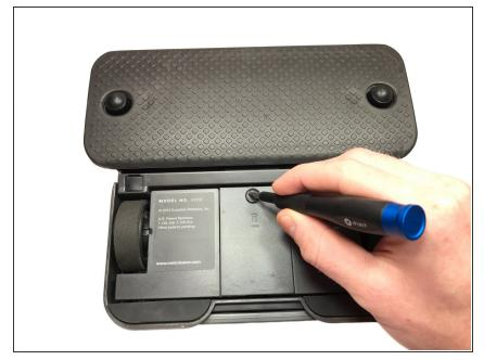
Remove the 4mm flathead screw on the battery cover.
