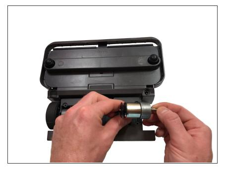
Flip the unit over and pull the motor out.
