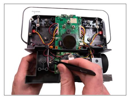
Using the blunt nose pliers, peel up the adhesive and feed the wires with adhesive through the opening.
