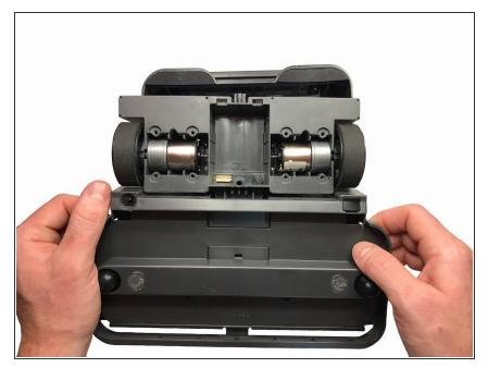
With the device upside down, pull up to separate the bottom from the top cover.
